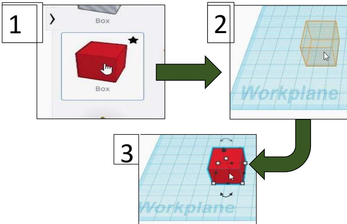
Fig 2.6 Steps for moving a shape
