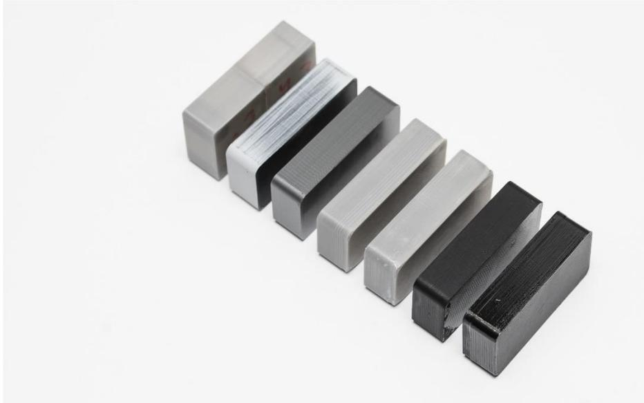
Fig. 3.1 Post processed FDM prints (from left to right): Cold welding, gap filling, unprocessed, sanded, polished, painted and epoxy coated.
