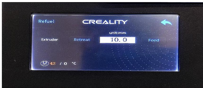
Fig. 2.29 (iii) Refuel option- Setting- Used to Retreat and feed the filament.
