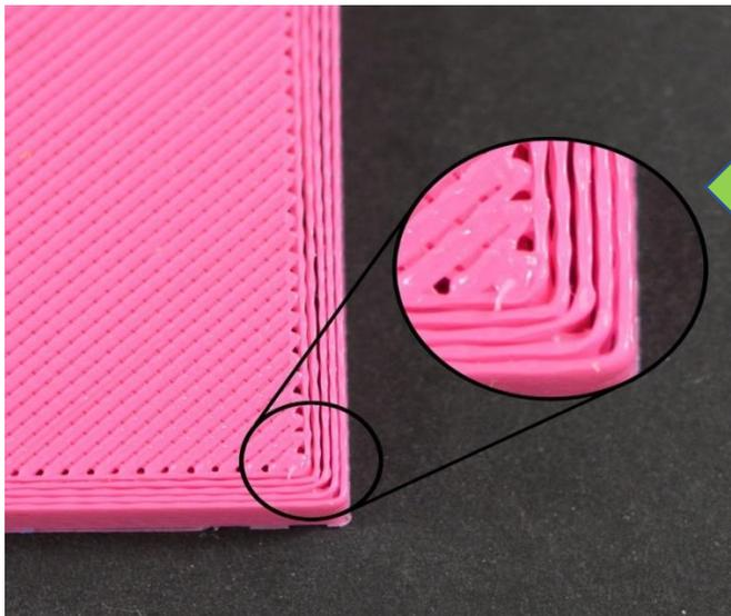
Missing layers due to improper discharge of filament through the nozzle.
