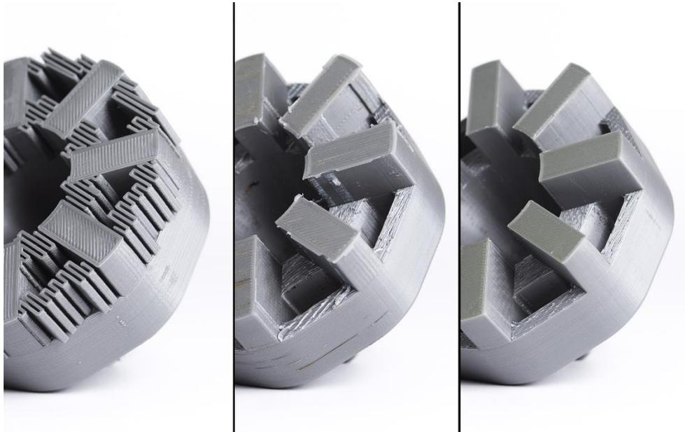
Fig. 3.2 Original print with support attached, poor support removal and good support removal (left to right)
