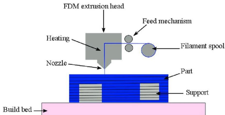
Fig1.1 Basic Procedure of FDM
