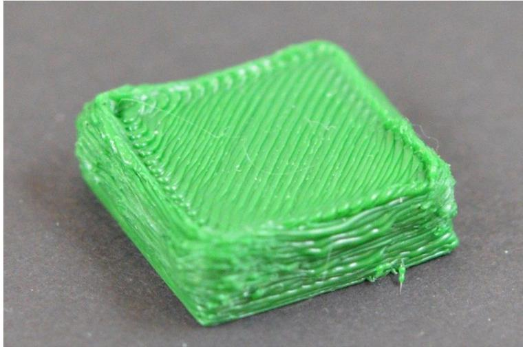
Fig. 2.34 Over- Extrusion
