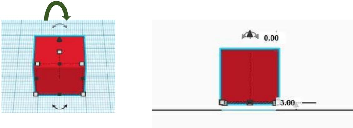
Fig 2.8 Moving a shape above or below the workplane
