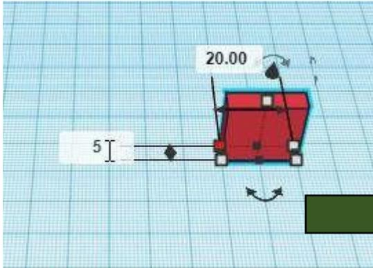
Once a shape is selected on the workplane, carefully click a small gray box to change a specific measurement of a shape by left clicking within the white text boxes that appear.
