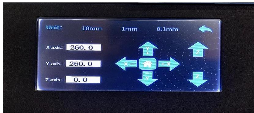
Fig. 2.29 (ii) Move Option in setting – Enable move the heat bed as per your preferences.
