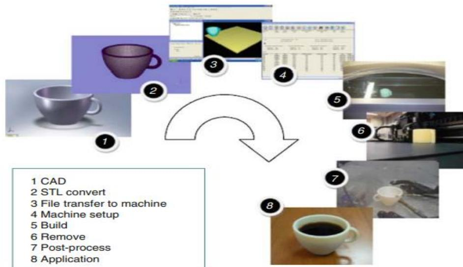
Fig 2.1 Generic Process of FDM
